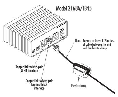
Figure 6. Connecting the ferrite clamp for 2168A/TB45 models
